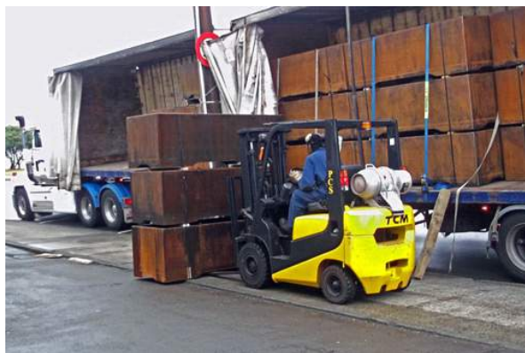
Large planters destined for Blenheim. Made using Corten weathering steel for a naturally rusting effect.
